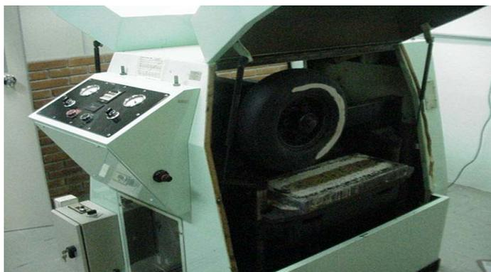
Figure 2. LCPC traffic simulator
