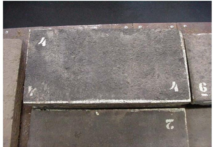
Figure 3. Specimens cored from full-scale test sections
