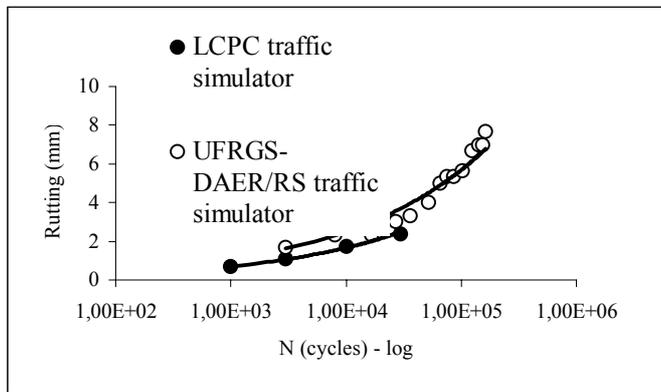
Figure 7. Comparison of rutting evolution using both traffic simulators
