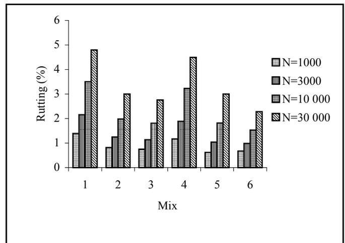
Figure 4. Laboratory tests results using LCPC simulator
