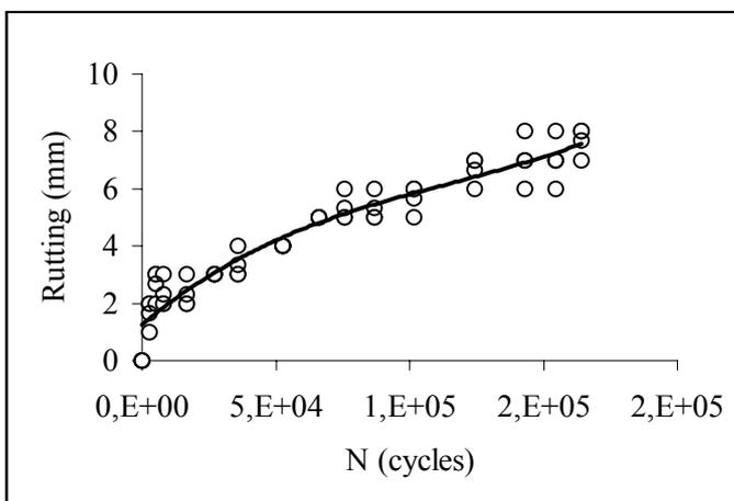
Figure 6. Rutting evolution in a test section loaded by UFRGS-DAER/RS traffic simulator
