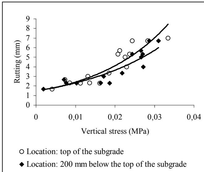
Figure 8. Rutting as a function of measured compressive stress
